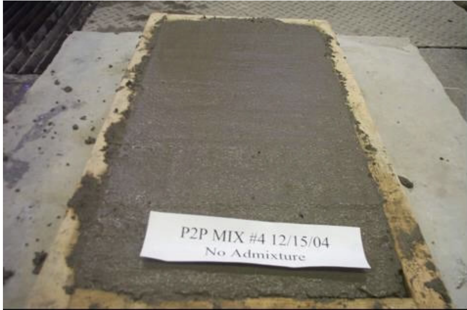
Figure 1 Finishability Test in Progress
