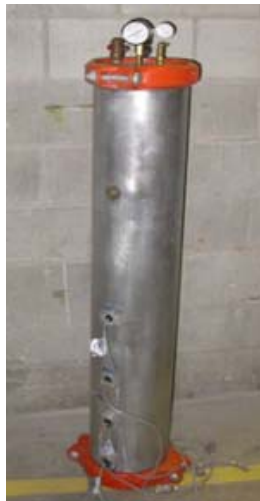
Fig. 1 – Sherbrooke pressure column enabling the measurement of form pressure of sections with up to 10 m in height
